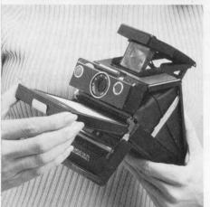
Insert a film pack, holding it by the sides, as shown.
