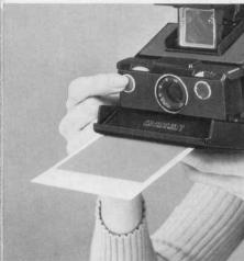
... until the picture comes out of the exit slot, and all camera sounds stop.
